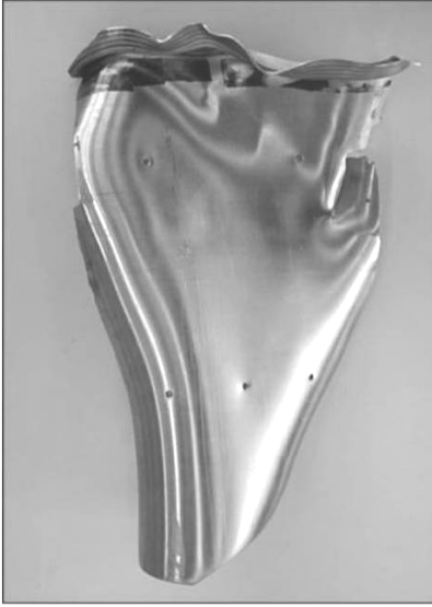
Crack after bunker test
